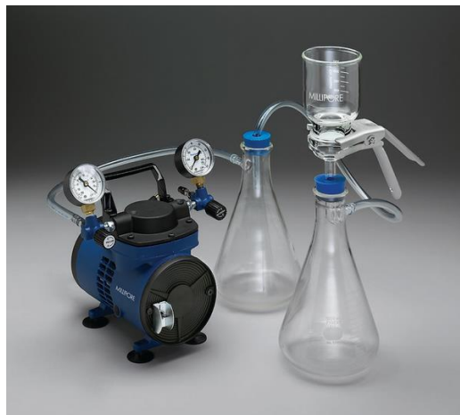
Figure 2 – Buchner filtration system with vacuum pump (credits: Merck Millipore)
